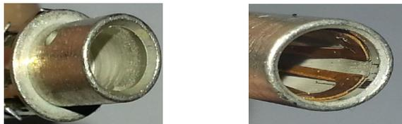
Actual images of stamped / crimped terminals from a EBS coiled cable used in a long combination experiencing some of the issues raised above
